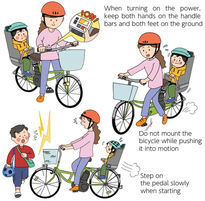
When turning on the power, keep both hands on the handle bars and both feet on the ground
